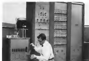
NEW AUTO-SORTER makes it economically feasible to search through large inventory of diodes for units with special characteristics. Auto-Sorter tests up to 25 diodes in batch.
